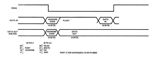
FIGURE 6. EXPANDED I/O TIMING DIAGRAM
